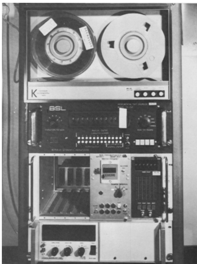
FIG. 1. Photograph of digital data station. The voltmeter is on the bottom of the rack, the clock scaler is on the right of the second row, and the master control module is next to it. The tape coupler is mounted below the incremental tape recorder. The indicative data are entered on the tape by the thumb wheel switches in the center of the tape coupler unit.
